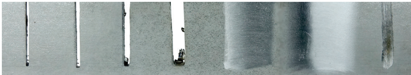
CUTTING WHEEL CUTTING WHEEL CUTTING WHEEL SNAGGING WHEEL BLENDING DISC SURFACE CONDITIONING DISC - MEDIUM SNAGGING WHEEL .035" 1/16" 1/8" 1/4" 36 GRIT 1/4"
