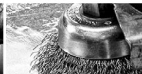
Rust / Oxide Removal
